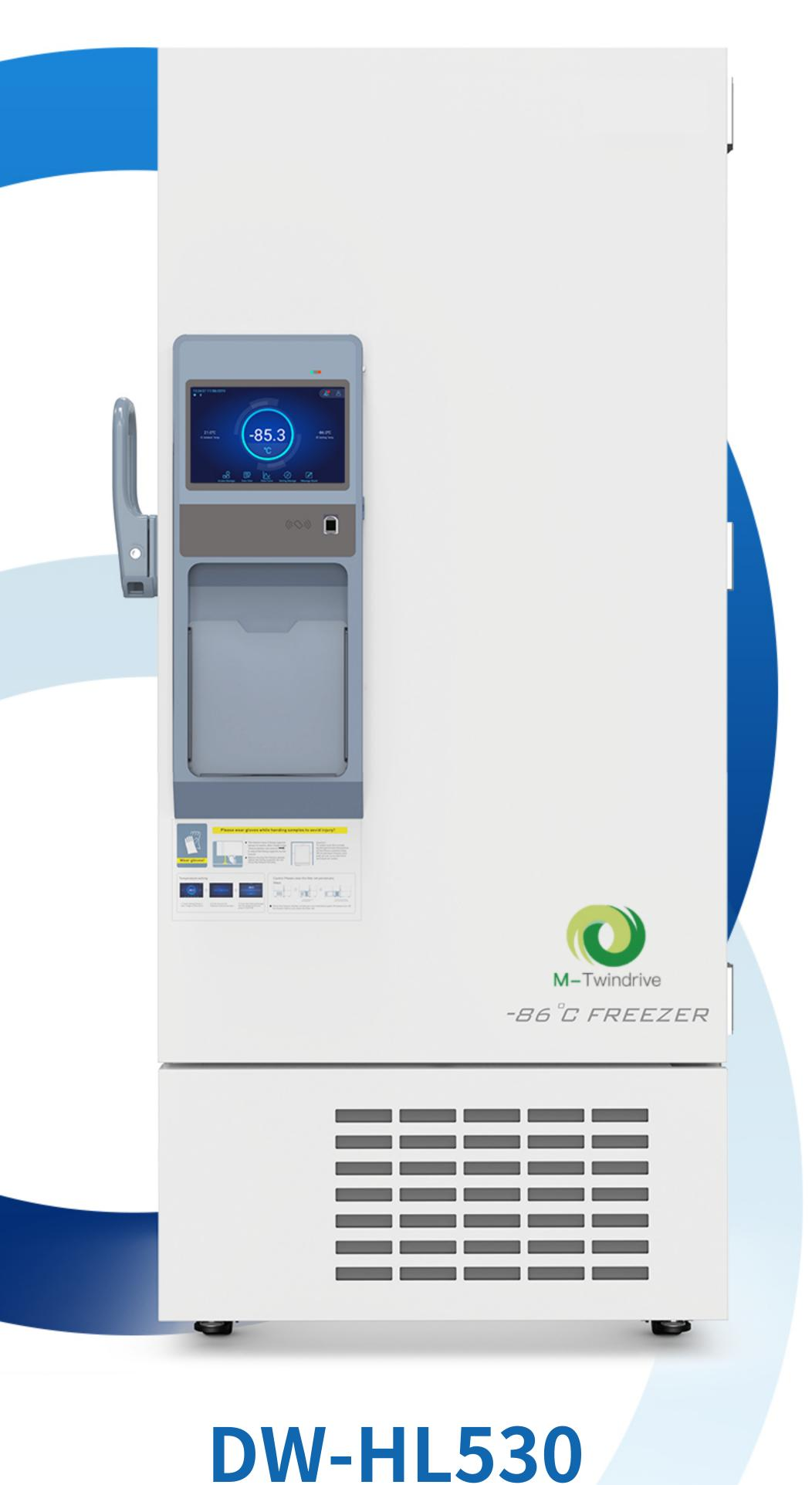
M-Twindrive -86°C Ultra Low Temperature Freezer built up by two independent refrigeration systems and the Dual Cooling System offers the highest level of protection, if one system unexpectedly fails the other can maintain the freezer around the -75°C. Valuable and irreplaceable samples can always be securely stored with the highest confidence even if the compressor fails.
